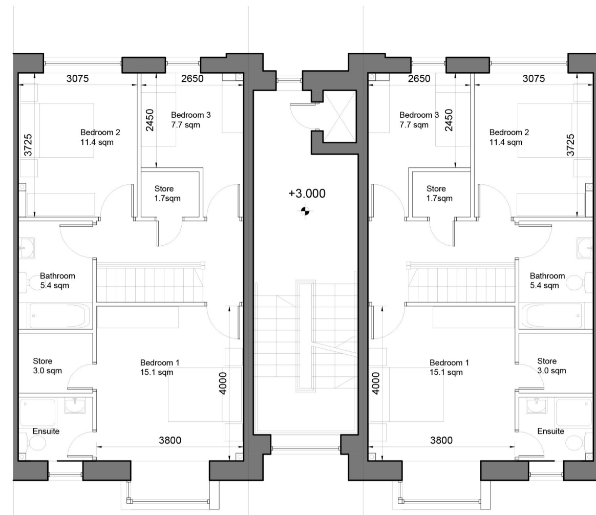
Typical Duplex Type 2A First Floor Plan
